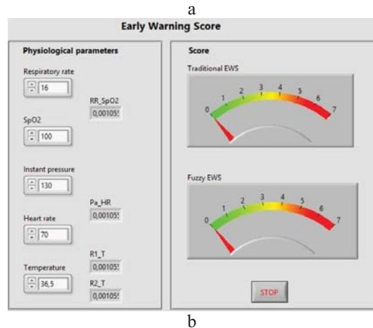
Fig.5. Implementation of the virtual biosensors for the estimation of medical precursors: a) Labview routine, b) front panel with aggregate scores and responses
